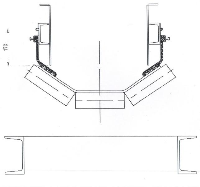
OFFSET MOUNTING USING CHANNEL
